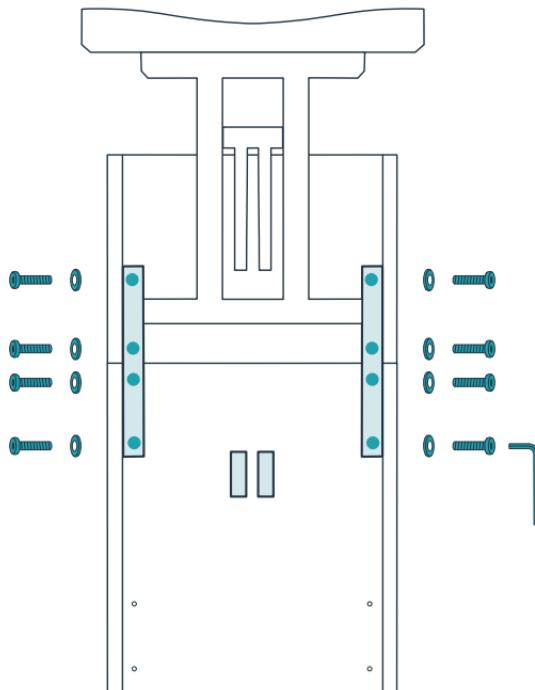
First, attach the angled support braces to the top platform, using four short screws and washers. Next, attach the angled support braces to the middle platform, using four short screws and washers. The mounting blocks on the middle platform should be on the side closer to the top platform. Wait until all the screws are in place before you tighten them.
