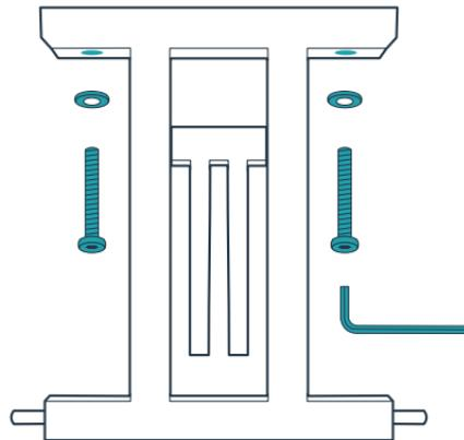
Attach the support leg foot to the support leg with two long screws and washers.
