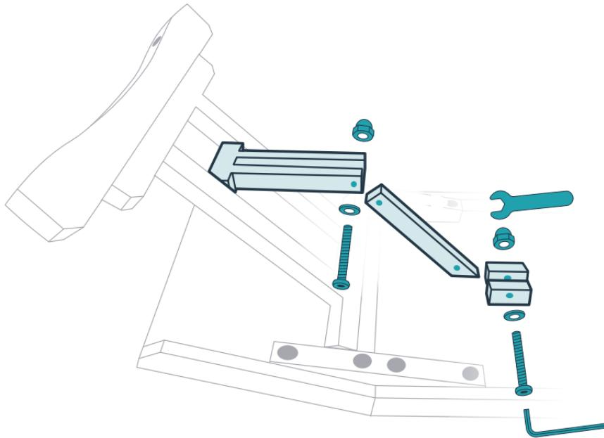
Attach the angled end of the leg brace extension between the mounting blocks on the back of the middle platform with a long screw, washer and cap nut. Attach the straight end of the leg brace extension between the two prongs of the leg brace with the remaining long screw, washer and cap nut. Before using the ramp, make sure all the screws are fully tightened.
