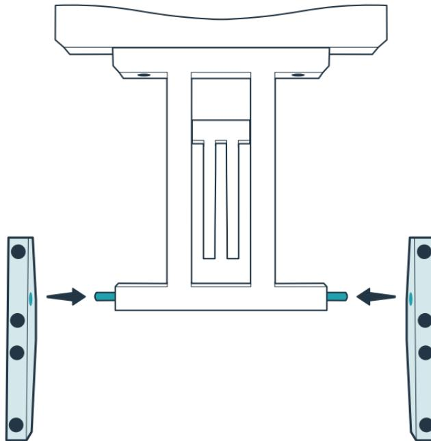
Fit the angled support braces onto the dowels at each side of the support leg.
