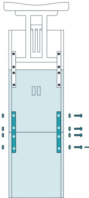
Attach the straight support braces to the middle and bottom platforms with eight short screws and washers. Wait until all the screws are in place before you tighten them.
