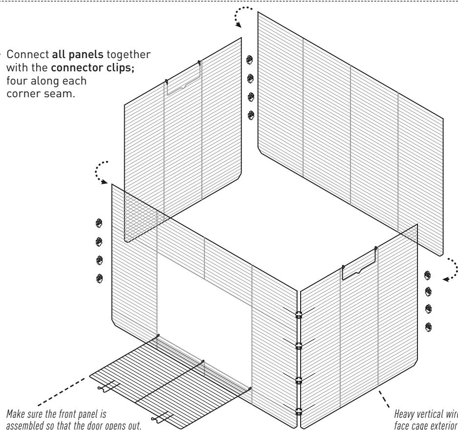
Make sure the front panel is assembled so that the door opens out.
