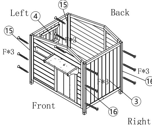
Fix ⑯\*2 Left iron wrap on ④ Left panel with screws, Fix ⑯\*2 Right iron wrap on ③ Right panel with screws.
