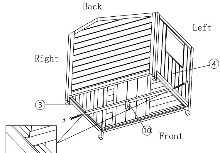
Fix ⑩ Support of bottom panel on ③ Right panel and ④ Left panel with screws.
