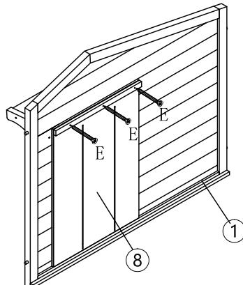
Fix ⑧ Door curtain on ① Front panel with screws.
