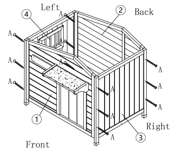
Fix ① Front panel, ② Back panel, ③ Right panel, ④ Left panel with screws.
