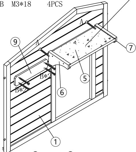
Fix ⑤ Door roof, ⑥ Left support of door roof, ⑦ Right support of door roof with screws.
