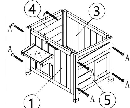
Fix ①Front panel, ③Back panel, ④Left panel, ⑤Right panel with screws.
