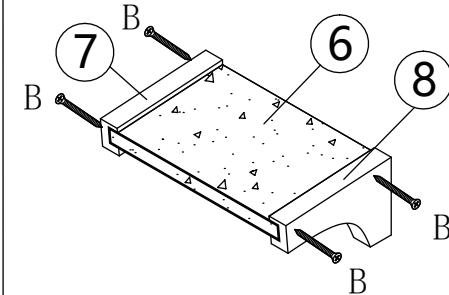
Fix ⑥Small roof, ⑦Left supporter, ⑧Right supporter with screws.
