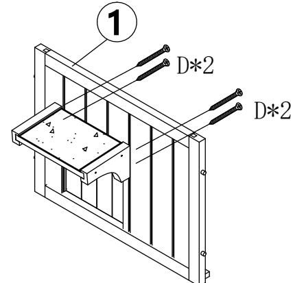
Fix the part of assembled Step 2 on ①Front panel with screws.
