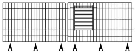
Attach the Velcro strap to the pen in the noted locations below. Wrap the lower strap underneath the bottom wire, and the upper strap over the top of the fourth wire from the top.
