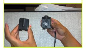
5. Remove the impeller gently—you will feel a slight tension as the magnet releases from the pump.
