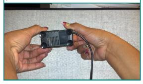
4. This is what you should see once the front/ bottom plate is removed. The next step is to remove the white fan piece called the impeller.
