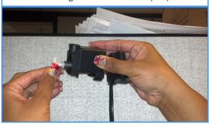
6. Clean the impeller and the "well" of the pump thoroughly.
