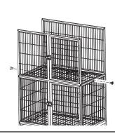
Slide the upper level side panels into place and secure with a long screw in all top and bottom corners.
