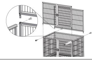
Slide the upper level front and back panels into place and secure with one long screw in each corner. Note: each corner screw will secure the intersection of three panels.
