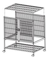
Slide the lower level side panels into place. Note: the track that will hold the mid-level floor is at the top and facing in. Secure the panels with one long screw in each bottom corner.
