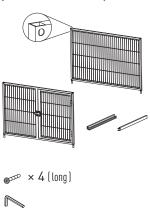
Guide the lower level front panel (with door) and back panel into the leg frames as illustrated. Note: the lower panels have openings at the top corners.
