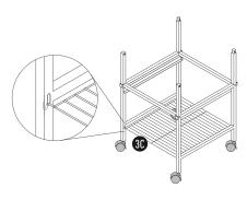
Locate the duplicate perch bar support (4L & 4R) posts. Insert the open end of the bar over the rounded back posts on the side left and side right frames.
