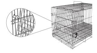
With the side panel caught on the loops, pull out at the top edge, push down on the main body top edge, and hook the side panel loop over the main body wire.
