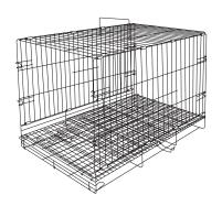
From the interior, pull the first side panel up into place. Allow the panel to catch on the two looped wires along each side of the main cage body.
