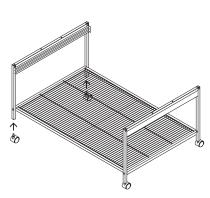
Flip assembled unit over and fully insert casters into frame legs.
