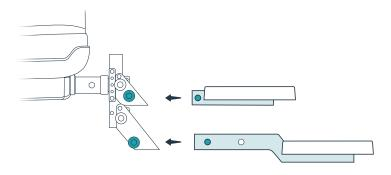
Insert each step into its bracket. Pull and release the red cap on each bracket to lock the spring pin into place. The lower step has two holes; for now, use the hole nearest the end.
