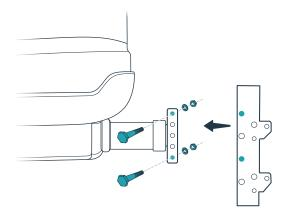
Line up the top hole on the hitch insert with the top hole in the vertical mount. Use two medium bolts, two small washers and two nuts to secure the insert to the mount.
