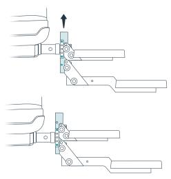
Check the position of the steps. If they're too low, you can move the vertical mount up so the lowest hole is lined up with the lowest hole in the hitch insert.
