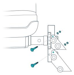
Use a short bolt, a small washer and a nut to secure each step bracket to the vertical mount. The brackets should be able to swivel up and down on the mount.
