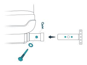
Slide the hitch insert into your vehicle's hitch receiver. Line up the first or third hole in the insert (depending on the length of your receiver) with the hole in your receiver. Insert the long bolt into the threaded hole and secure it with the large washer and retaining clip.
