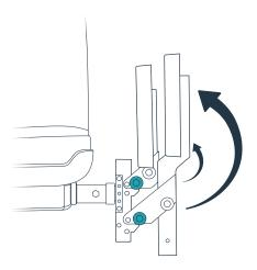
Stow the hitch step before driving. On the lower step, pull the red cap and slide the step in so the spring pin locks into the second hole. To fold each step, pull the black cap, fold the step up and release the cap to lock the spring pin into the upper hole.
