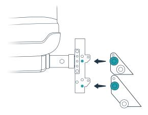
Slide each step bracket over the vertical mount. Pull and release the black cap on each bracket to lock the spring pin into place.
