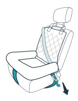
Loop the strap over your vehicle's headrest and then reach under the dog bed to push the white seat anchor tube between the seat back and seat bottom. (The large dog bed has two headrest straps and two seat anchor tubes.)
