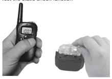
Screw the wires of the test bulb around the contact probes of the receiver. Turn on the remote transmitter by pressing the Mode button for 1 seconds, switch to Shock mode and then press the UP/DOWN button to adjust the intensity level. Press the Y button and the test bulb will flash, signifying that the Shock function works. Please make sure that the Shock level is well above 0 when testing the function.
