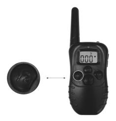
Use a toothpick to poke through the Reset hole of the receiver collar and press the inner button gently. Red light will begin to flash.
