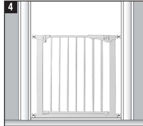
**4** Center the gate in opening with bottom rail resting on floor. Gaps on each side should be equal. **IMPORTANT:** The gate must be level and straight up and down, otherwise the gate's door will not function properly.
