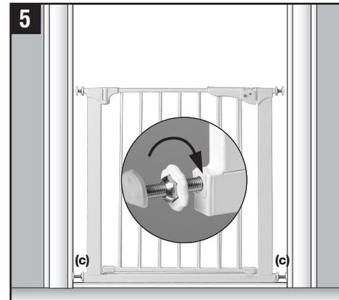
**5** Pull out the two bottom spindles (c) until they touch the mounting surface and rest on top of floor molding (if applicable). Tighten handwheels TOWARD GATE FRAME as tightly as possible. Each spindle adjusts individually and may be extended to varying lengths to allow for molding, uneven walls, etc.
