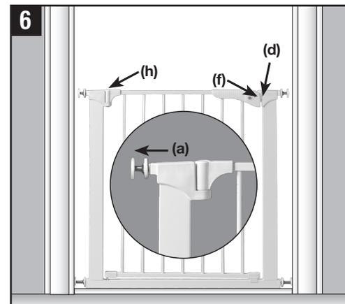
**6** Close walk through door so pressure plate (f) is aligned with pressure hinge (d). Pull out the top spindle (a) on the hinge side (h) until it touches the mounting surface. Tighten handwheel TOWARD GATE FRAME.
