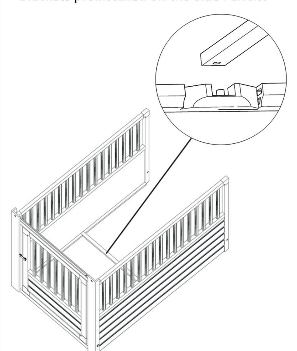
Step 4: Install the floor panel (4).
