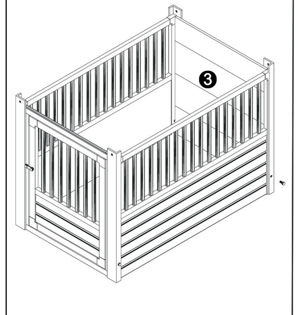
Step 6A: (for L and XL only) Insert the Side Wall Pin into the bracket preinstalled on the upper edge of the Side Wall Panel.
