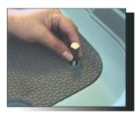
1. Push "stainless steel bolts" through four holes in bottom of tub.
