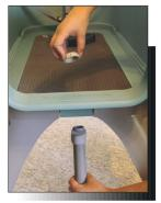
8. Attach drain hose by pushing through large hole in rear of tub and securing with threaded cap.
