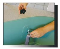
Place thick washer over end of eyehook and push through sidewall of tub, spin on five star knobs firmly.
