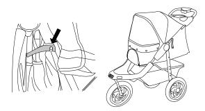
**2. INSTALLING THE FRONT WHEEL:** Place the wheel axle at U tube groove and attach hook-shaped gasket. Use wrench to tighten the nuts on both sides. Make sure the gasket is tightened by the two nuts.
