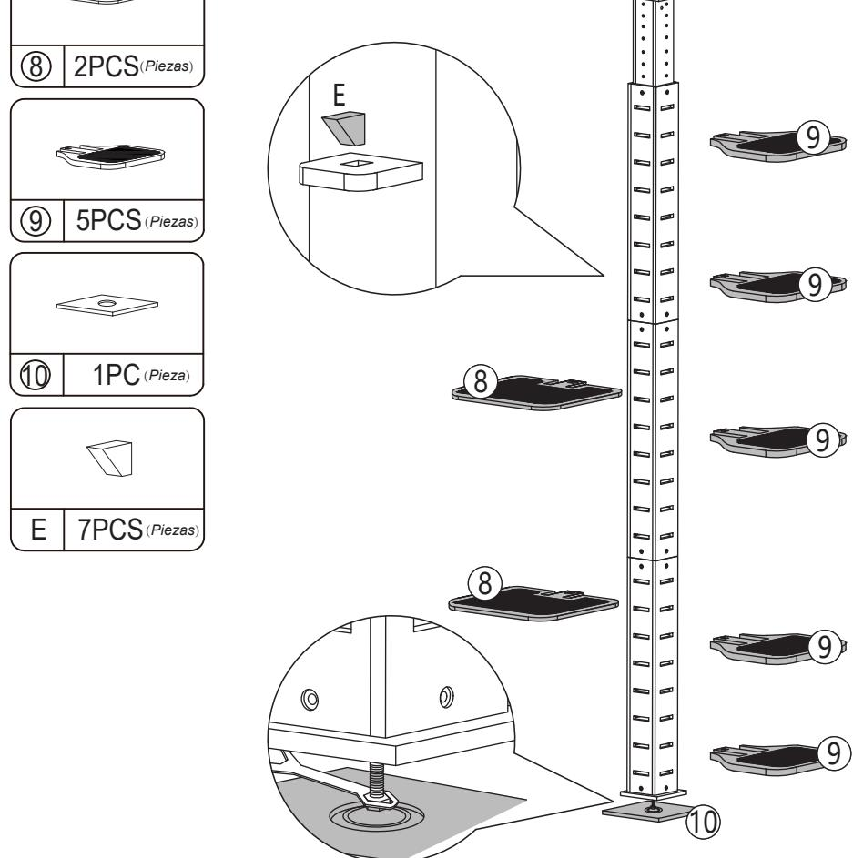
**By rotating the foot cup, the column length can be adjusted slightly.**
