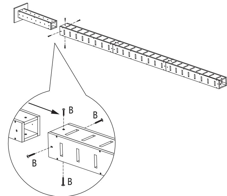
**You can adjust the column length by screwing into different holes according to your needs.**
