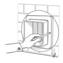
Mark the position of the two screw holes required to mount the external frame and then drill appropriate holes in the wall.
