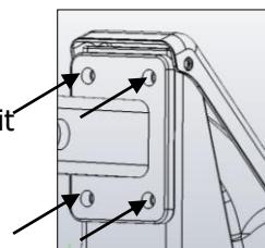
c. Loosen and remove the 4 screws holding the receiver bar to the tower assembly of the TWISTEP with the included Hex Key.
