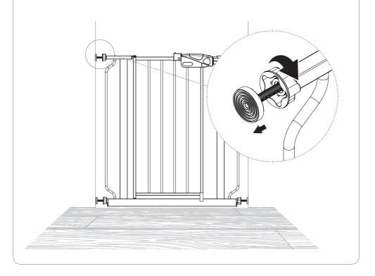
**NOTE:** It may be necessary to hold the *threaded spindle rods* or *rubber feet* while rotating the *adjustment wheels* to ensure the entire unit does not rotate.
