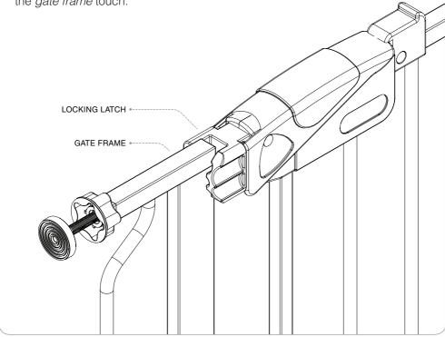
**NOTE:** The gap between the gate and wall should not exceed more than 2 inches. Make the appropriate adjustment to ensure you have installed your gate safely.
