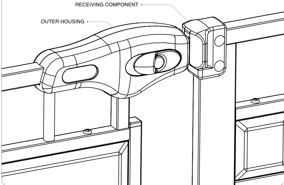
**NOTE:** The gap between the wall and gate should not be more than 2-1/2 inches. Make the appropriate adjustment to ensure you have installed your gate safely.
