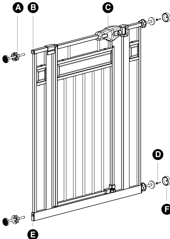
**A** **Threaded Spindle Rods
