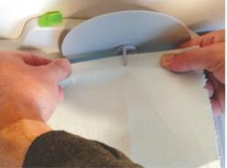
**Step 5:**Press the **Pad Advance** button on the Control Module to roll up the paper. If the Pad Roll slips out of the clips, re-insert the Pad Roll into the clips.
