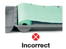
**Step 4:**Tuck paper into upwardly facing clips on each end of the Take-up Rod.
