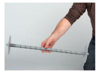
**Step 2:**Drop take-up assembly into waste area near Control Module. Gear Cap will mate to Control Module gear:
