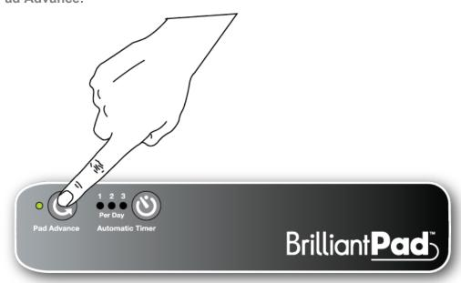
PRESS AND HOLD Pad Advance button to advance pad. Release button to turn off motor.
