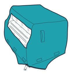
Continue pulling the cover over the frame until the rectangular bottom panel of the cover lines up with the bottom of the frame.
