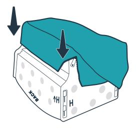
Set the plastic frame upside down. Open the zipper at the back corner of the fabric cover and slide it over the bottom of the frame. The zipper should line up with the corner of the frame marked "H".
