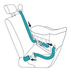
Pass your vehicle's seat belt through the slit at one side of the safety seat, through the seat belt tether loop, through the slit on the opposite side of the safety seat and buckle it.
