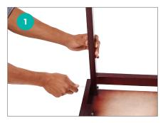
**STEP 1** Place the support ladder (#6) on the short panel (#4), lining up the 2 screw holes on the support ladder with the 2 threaded holes on the free end of the short panel. Insert screws (C) and washers (F) on each side, then tighten screws with nuts (G) using the included allen key (E). Use pliers if needed.
