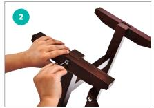
**STEP 2** Locate the 2 support feet (#9) to connect to the support ladder. Align the holes on the support feet with the holes on the bottom of the support ladder. Insert screw (A) and tighten fully.
