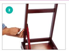
**STEP 2** The 2 angled braces (#7) act as support beams to secure the support ladder (#6), so have them handy. Align angled brace with the threaded hole on the inside middle of the support ladder and the threaded hole on the inside middle of the bent brace. HINT—This is the hole we left open in part 2. Insert screws (D) and washers (F), but DON'T TIGHTEN YET.
