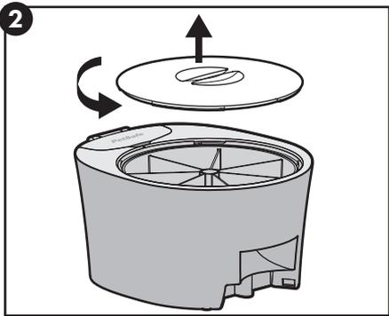
2. Unlock and open the lid by rotating counter-clockwise and lifting up.
