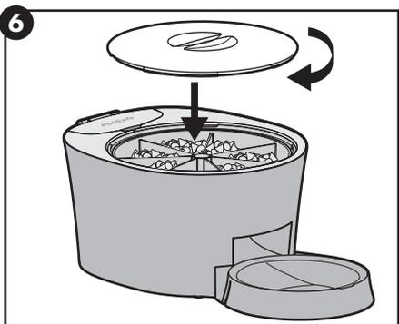
6. Replace the lid and turn clockwise to lock into place.
