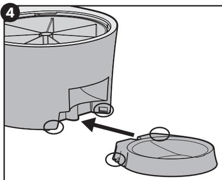
4. Attach the bowl by inserting the side tabs into the slots on the bottom front of the feeder.
