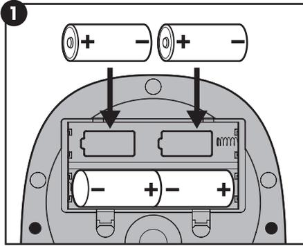
1. Insert four D-cell alkaline batteries into the battery compartment located on the bottom of the feeder.
