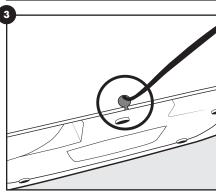
4. Remove the extra slack from the cord and push the rubber gasket firmly into the hole.
