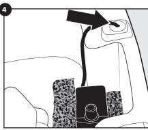
5. Attach the rubber connector to the pump tube if it is not
