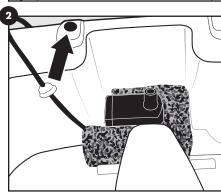
3. Once the pump is securely in place, feed the cord through the hole on the back of the bowl and out the notch on the bottom of the bowl.
