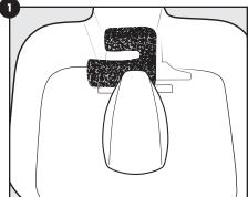
2. Place the pump inside the foam filter on the bottom of the bowl. The cord will be closest to the hole on the back of the bowl. Press down on the pump to engage the suction cups.
