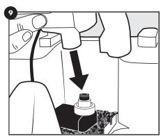
Align the bottom tab of the filter housing with the raised notch. The flat side (Side B) of the filter housing will be facing the front of the bowl.
