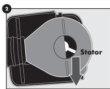
3. Use a fingernail to pull out the impeller, which is held in place magnetically. Clean the pump parts with warm water and soap, then reassemble.
