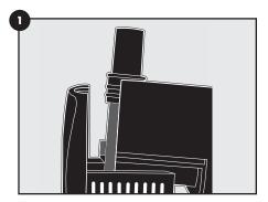
Remove the yellow, teardrop-shaped stator by pulling up on the small tab.
