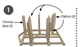
Insert the Chimney Base (9) into the top horizontal slot (nearest to the triangle "roof frame" section of the form) of a Tower Frame (1).
