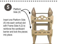
Repeat Steps 4 & 5 on the other side of the Tower Frame (1) using the shorter Frame Side B (2) to align with the lower platform set. Remember to lock into place using Platform Side (4) for each Platform level.
