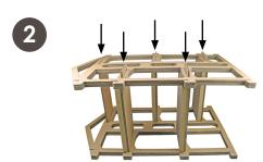
Carefully attach the other Tower Frame (1) to the other ends of the Chimney Base (9) and Platforms (8). (Caution: The frame may be unstable during assembly. Take care not to bend or apply weight onto the frame during this step.)
