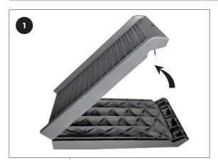
**STEP 1**Take out the hook and unfold ramp.
