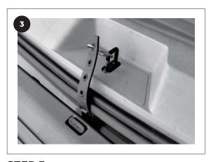
**STEP 3**If used on the rear entrance of a van or SUV, attach the security strap to the floor door latch, as shown.
