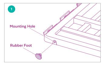
**STEP 1** Connect the rubber feet to each panel. (2 rubber feet on each panel)
