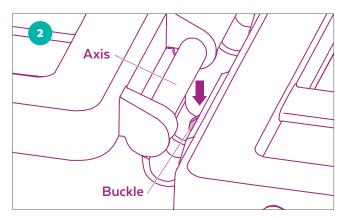
**STEP 2** Connect the panels by pressing the axis downward into buckle to snap it into place.
