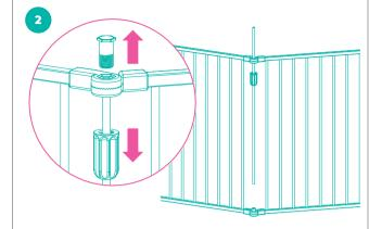
**STEP 2** Remove the lock bolt on the top opening of the upper connectors and then remove the pipe holding the panels together. Repeat for each side.
