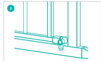
TO CLOSE Pull the door shut and make sure the top latch closes. Move the bottom lock on the side occupied by your pet (aka their new chill spot) to the down position.
