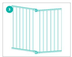
**STEP 3** Position the enclosure in your preferred configuration and bring the open ends together at the plastic connectors. Sit. Stay. We're halfway there!
