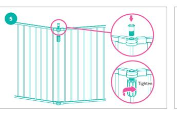
STEP 5 Locate the Lock Bolt. Insert it through the top opening in STEP 6 Work your way around the enclosure, tightening the lock the upper connectors. Move the lock nut up to the joint created by unuts between every panel to lock the enclosure in place. Woof. the upper connectors and tighten it. From gate to pen, just like that! Now it's really time for a treat break.
