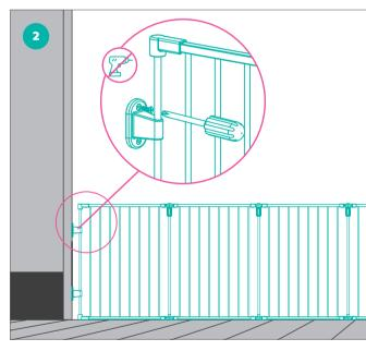
**STEP 2** Fix one of the top wall mounting brackets (attached to the gate) to the wall using a Phillips head screwdriver and two screws. Repeat for the other top wall mounting bracket, making sure the gate is even across the opening.
