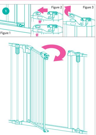
TO OPEN Make sure the base locks are in the horizontal position (figure #1). Pull the spring lock away from the easy open latch (figure #2) and lift the lock lever upwards (figure #3) at the same time to release it. Then, pull the gate open. Neat, amirite?
