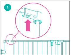
**STEP 1** Locate the bars with the wall mounting brackets attached to both ends of the gate. Press the spring buttons down on the connectors, remove each end bar and store them for later use.
