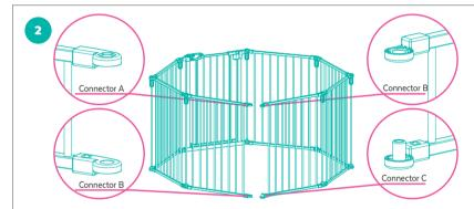
STEP 2 On the top bar of one side of the gate, install Connector A. Install (1) Connector B on the bottom bar. On the opposite side, install (1) Connector B on the top bar. Install Connector C on the bottom bar.
