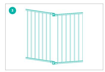
**STEP 3** Set aside the panel, pipe and hardware. Then, close the open ends of the enclosure. Full circle...or whichever shape you choose!
