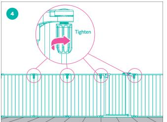
STEP 4 Tighten the lock nuts between every panel to lock the gate in place. Time for a treat break!
