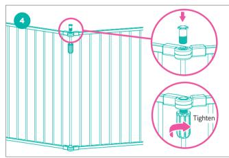
**STEP 4** Replace the pipe, lock nut and lock bolt. Then, tighten the lock nut to secure the enclosure again.
