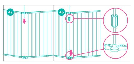
STEP 4a Locate the Fine Connecting Pipe and Lock Nut. Insert the pipe through the upper connectors on the open ends of the gate. 4b Thread the lock nut onto the pipe between the top and bottom bars with the flat side facing up. Then, guide the pipe into the circular housing on the bottom connectors.
