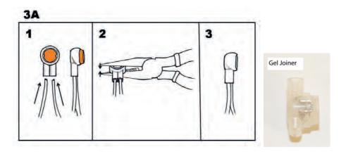
Note: Pliers should be used to push down fully the RAISED part of the wire connectors to ensure that the wire insulation is pierced so the radio signal can run through the connector.
