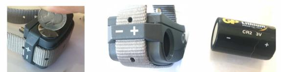
Prepare the receiver collar by removing the silver cap on the side of the receiver and insert one CR-2, 3 Volt battery. The positive + must be facing back out toward the silver cap, or follow plus/minus symbols printed on receiver collar (see image above). Replace the silver cap once you have installed the battery correctly. Your receiver is set to Level One. We recommend you use this level. Only a few dogs may require higher levels. Go to pg 11 in the Product Manual for more information.
