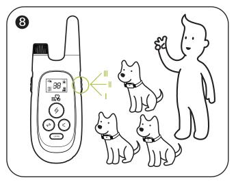
**Channel switching:** it is possible to train 3 dogs at the same time. Toggle the CHANNEL SWITCH to select which dog to train.
