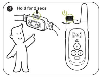
Turn on the collar: hold the ON/OFF BUTTON for 2 seconds.
