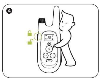
Unlock/Lock the remote control keypad: toggle the KEYPAD LOCK down to unlock, and up to lock.
