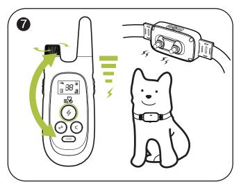
Static intensity adjustment: press and hold the LEVEL BUTTON while rotating the ON/OFF SWICTH to adjust the static intensity.
