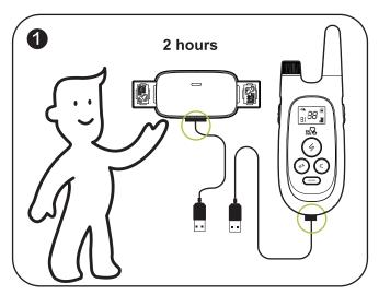
Charge the collar and remote control with the included USB cable. Charging takes approximately 2 hours respectively.
