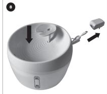
STEP 8 - INSERT THE LEAF UNIT INTO THE HOLE AND PLUG IN
