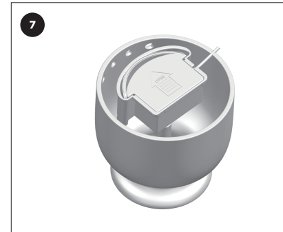
STEP7- INSTALL THE PUMP RACK ON THE COVER AS A WHOLE
