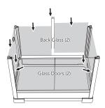
4. When all the four sides have been installed, place the top frame without the top metal ventilation mesh. Make sure that the top frame sits in properly.
