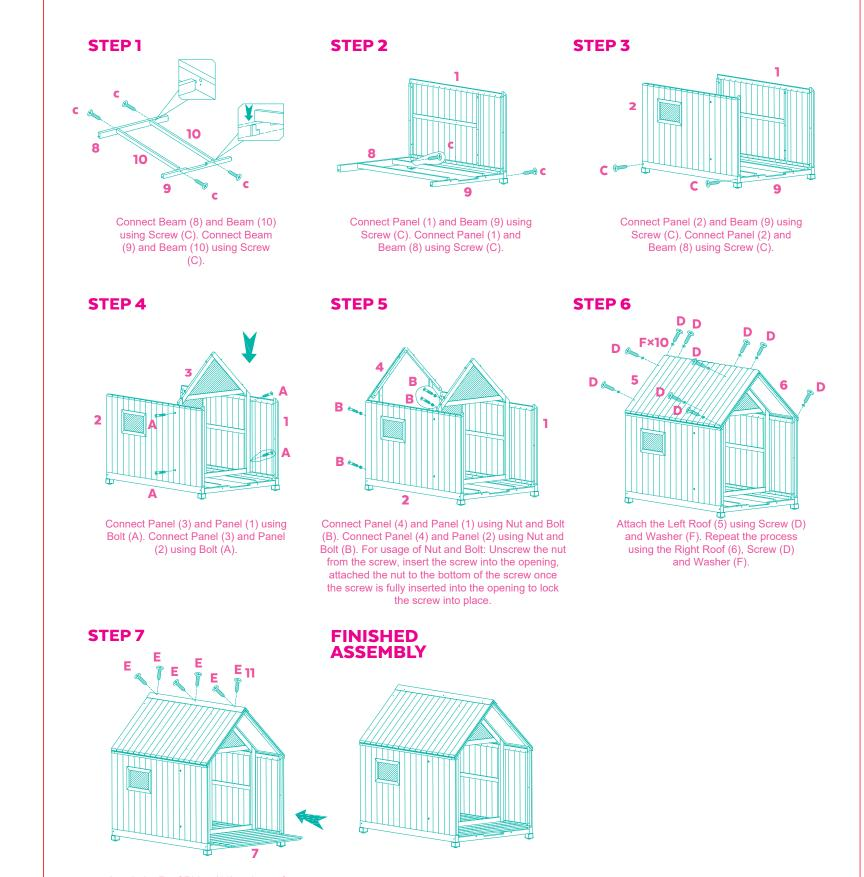
Attach the Roof Ridge (11) to the roof using Screw (E). Insert the Floor (7).
