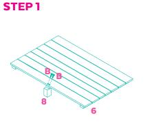
Fix the Base Support (8) to the underside of the Floor (6) using Screw (B).
