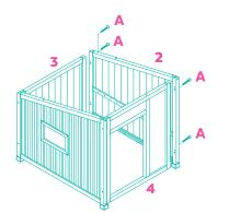
Connect Panel (2) and Panel (3) using Screw (A). Connect Panel (2) and Panel (4) using Screw (A).
