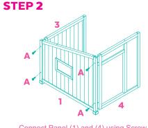
Connect Panel (1) and (4) using Screw (A). Connect Panel (1) and (3) using Screw (A).
