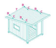
Attach the Roof (7) using Screw (B) and Washer (C).
