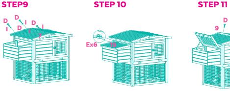
Attach the Left Roof (7) using Screw (D) and Washer (I).
