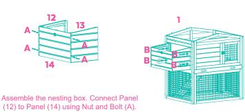
(12) to Panel (14) using Nut and Bolt (A). Connect Panel (13) to Panel (14) using Nut and Bolt (A). For usage of Nut and Bolt: Unscrew the nut from the screw, insert the screw into the opening, attached the nut to the bottom of the screw once the screw is fully inserted into the opening to lock the screw into place.
