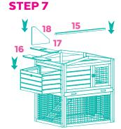
Insert the Floor (16), (17) and Partition (18) into the nesting box. Insert the roosting bar (15) into the house.
