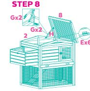
Assemble the Roof (8). Connect the hinged roof to Panel (2) using Screw (E). The hinge should be attached to the outside of panel. Connect Hinge (H) to roof and Panel (2) using Screw
