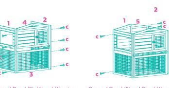
Connect Panel (3), (4) and (1) using Screw (C). Connect Panel (3), (4)
