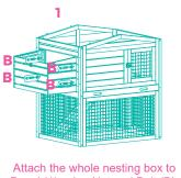
Panel (1) using Nut and Bolt (B).
