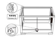
1. Install the threaded metal tubes provided to the base. Frist Check the Numbers and Arrow marks on the
