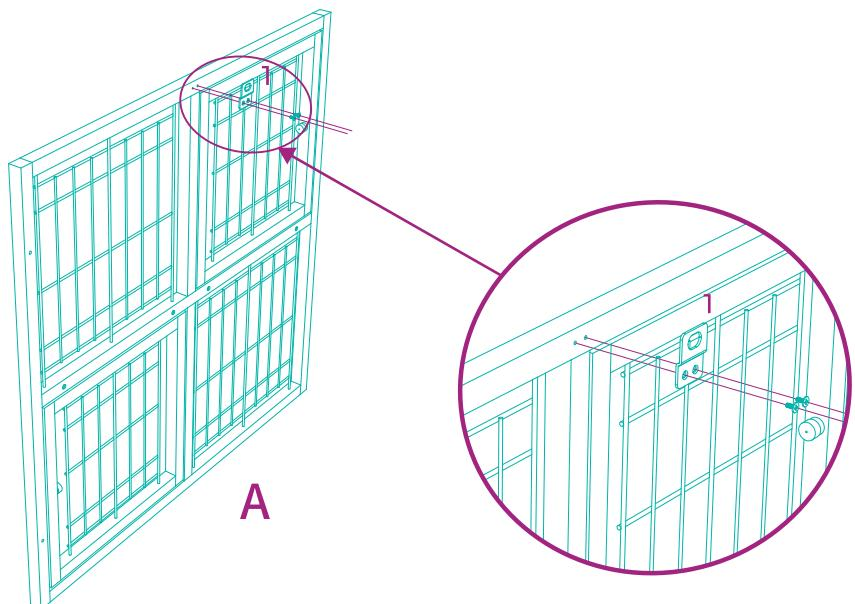
**STEP 1** Assemble the metal lock on the panel A as shown.
