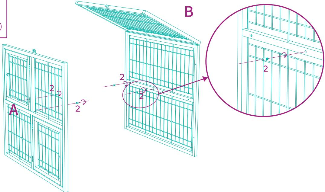
**STEP 2** Insert metal studs on the inside of panel A and of panel B as shown. The studs will hold the shelf board, panel E.
