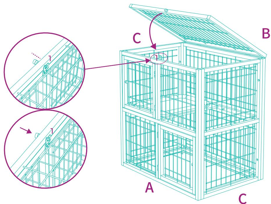
**STEP 5** Pull out the button on the roof, then push it to insert into the metal lock (1) to lock.
