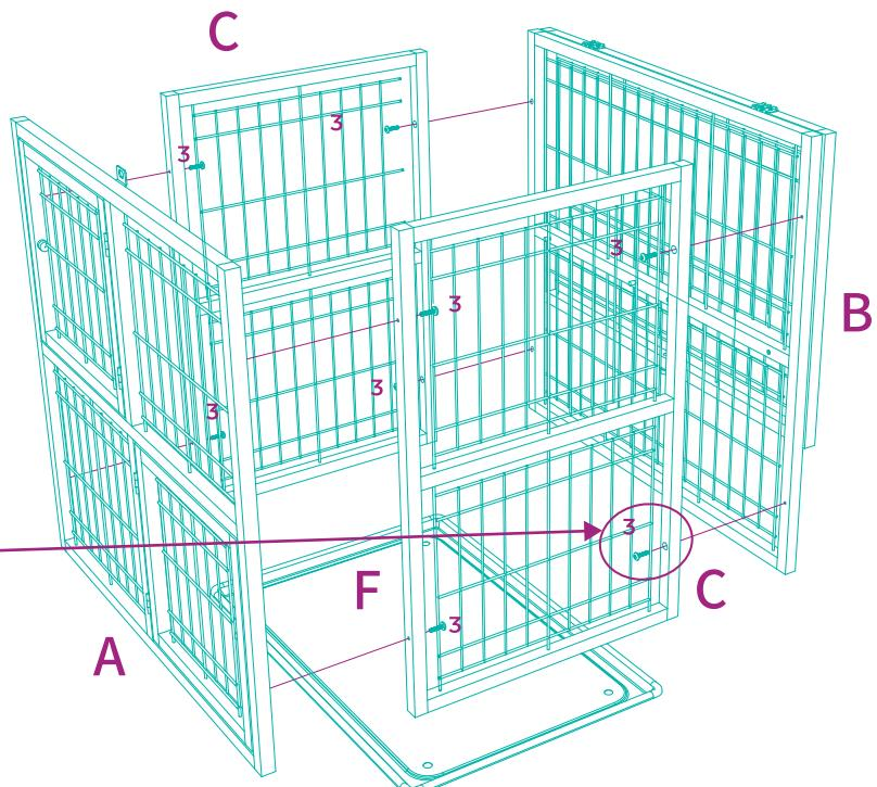
**STEP 3** Determine location of the playpen, place the plastic tray F in that location. Assemble panels A, B and C around the plastic tray F (as shown). Screw panels A, B and C together using screws (3) and the wrench (4).
