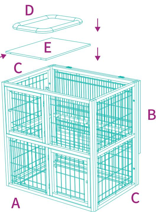
**STEP 4** Place the shelf board E on the metal studs, and then put the cushion D on top of the board.
