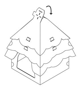
Step 10 Reinforce connections by placing Clear Stickers (J) over the tabs
