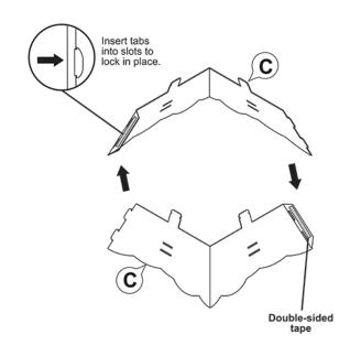
**Step 5**Connect **Middle Branches** to **Completed Panels** by folding in sides and inserting tabs into slots as shown.
