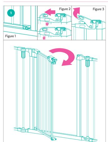
**TO OPEN** Make sure the base locks are in the horizontal position (figure #1). Pull the spring lock away from the easy open latch (figure #2) and lift the lock lever upwards (figure #3) at the same time to release it. Then, pull the gate open. Neat, amirite?
