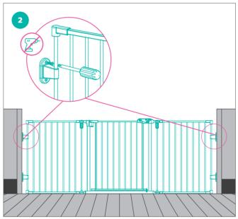
**STEP 2** Fix one of the top wall mounting brackets (attached to the gate) to the wall using a Phillips head screwdriver and two screws. Repeat for the other top wall mounting bracket, making sure the gate is even across the opening.
