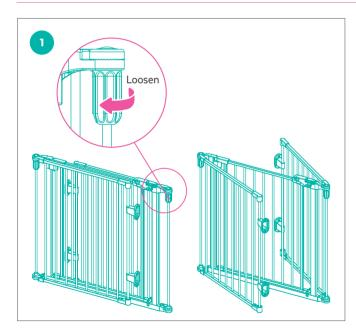
**STEP 1** Bring the gate to the installation area. Loosen the lock nuts on both sides of the door panel to allow the gate to unfold freely. Do not fully remove the lock nuts. Unfold the gate and set it up in the installation area. Pat yourself on the back!
