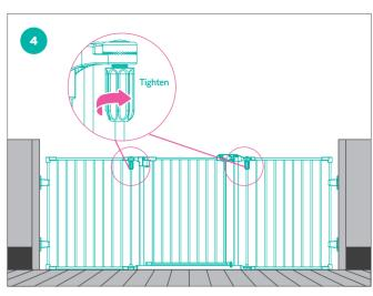
**STEP 4** Tighten both lock nuts on either side of the door panel to lock the gate in place. Time for a treat break!
