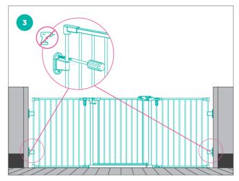
**STEP 3** Straighten the bottom of the gate to make sure it isn't leaning, i.e. tipping forward or backward, then repeat the installation process for both bottom wall mounting brackets.
