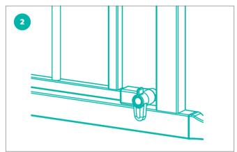
**TO CLOSE** Pull the door shut and make sure the top latch closes. Move the bottom lock on the side occupied by your pet (aka their new chill spot) to the down position.
