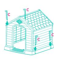
STEP 3 To install the side panels, slide them into the respective openings on the roof and back panels.
