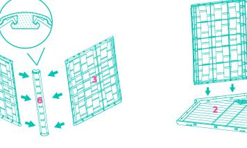
STEP 5 Attach the all panel using screw (D).
