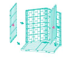
STEP 6 To install the bottom panel (5) line it up to the base of the dog house, then insert the plastic feet (A) into the notches on the bottom panel and attach using screw (E).
