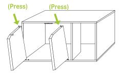
Orient door properly as shown and align bottom pin. Press on spring loaded top pin and insert.
