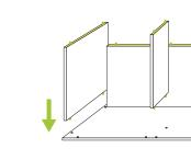
Align vertical zBoards to horizontal zBoard as shown. Press down firmly.
