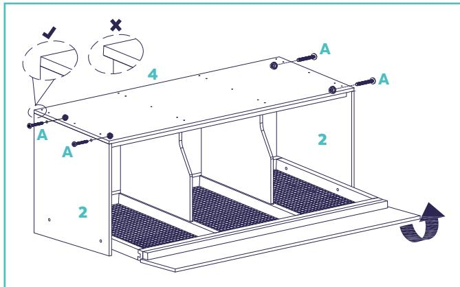
**Step 3.** Assemble Roof (4) to Panel (2) using Nut and Bolt (A).
