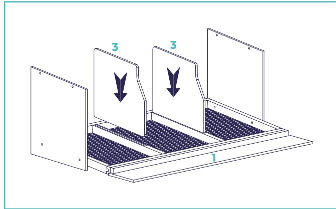
**Step 1.** Attach Panel (2) to Floor (1) using Nut and Bolt (A).
