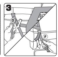
Pull top headrest straps (D) tight on both sides. Pull both both under-seat straps (F) tight.
