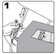
Orient the barrier so the Kurgo logo is facing the back of the car. Remove the driver's seat headrest. Slide the inner headrest column through the inner D-ring (A). Slide outder D-ring (B) through the outer vehicle headrest post. Repeat on the passenger side headrests.
