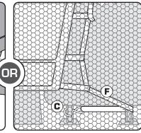
Option B: Run the under-seat straps (F) around the outside footing of each seat and secure the under-seat hook (C).
