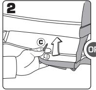
Option A: Clip the under-seat hook (C) to the underside of the front seat's base plate or springs.
