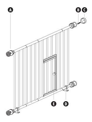
A Threaded Spindle Rods w/Adjustment Wheel Gray = #14016
