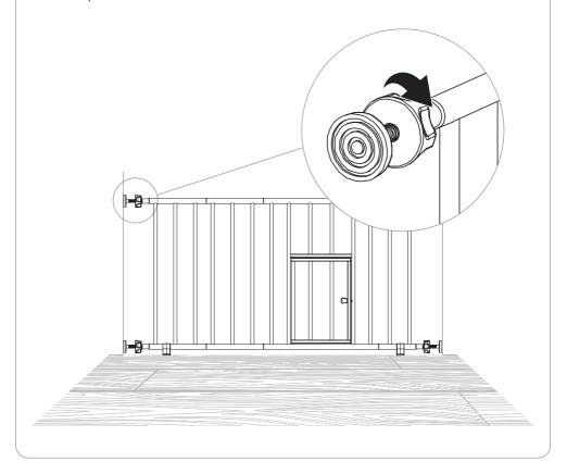
**NOTE:** It may be necessary to hold the *threaded spindle rods* or *rubber feet* while rotating the *adjustment wheels* to ensure the entire unit does not rotate.
