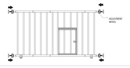
**NOTE:** The ends of the gate frame are not threaded. The *threaded spindle rods* should slide into the end of the frame tubes without any resistance.
