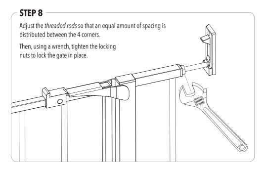
**NOTE:** The maximum length of the exposed threaded rods should not exceed 2.5 inches.
