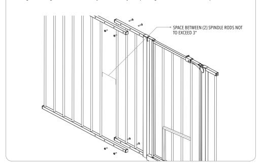
**NOTE:** You must use two sets of *double-ended screws* on top, and two sets of *double-ended screws* on the bottom.
